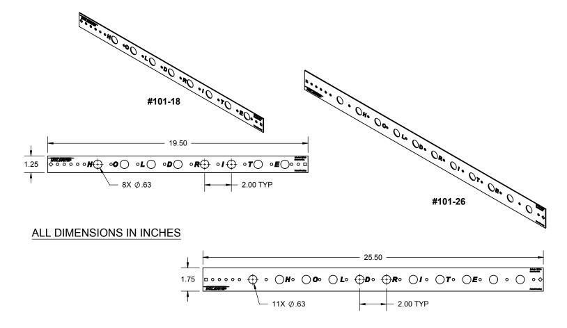
The HOLDRITE #101-18 & #101-26 is a Copper-Bonded™ steel brackets with 5/8" holes on 2" centers to support 1/2" copper tubing. The #101-18 & #101-26 position copper water supplies for sinks, water closets, and other fixtures. When soldering, heat the pipe, not the bracket.
