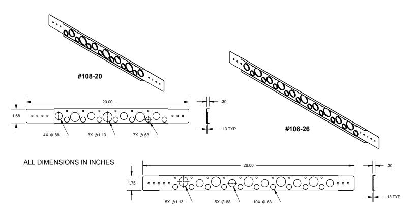
The HOLDRITE #108-20 and #108-26 are Copper-Bonded<sup>™</sup> steel brackets with holes for 1/2" pipes on 2" centers, holes for 3/4" and 1" pipes on 4" centers. Featuring a rolled-edge for added strength, and extruded holes for easier soldering. The #108-20 & #108-26 are designed to positions copper water supplies for urinals, lavatories and other fixtures. When soldering, heat the pipe, not the bracket.
