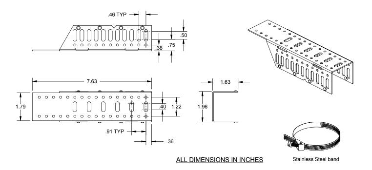
The HOLDRITE® #115 and #115-C (Copper-Bonded<sup>™</sup>) are steel brackets designed to position water supply lines off the vent or waste pipe in chase walls. Supports 1/2" through 2" pipes both vertically and horizontally. Packaged with self-locking stainless steel band, screws, metal clamps, and self-adhesive isolating felt. Excellent for pre-fab applications. Supports piping prior to wall framing. Heat the pipe, not the bracket when soldering the #115-C version.
