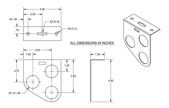
The HOLDRITE® #121-O is a 20 gage galvanized steel bracket that supports up to three lines of 1/2", 3/4" or 1" Copper, PEX or CPVC tubing. The hole pattern on the 90° base allows for attachment to any flat surface. The bracket can also be suspended by 3/8" threaded rod.
