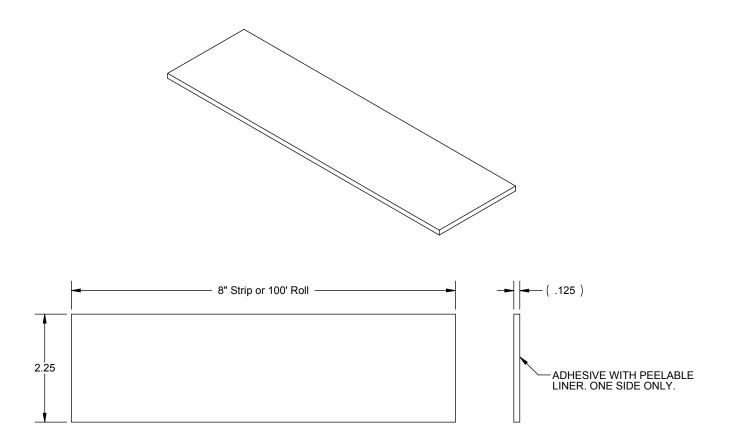
Felt 8 and Felt 100 HOLDRITE Isolating felt for use in eliminating dissimilar metal contact and provides minimal sound vibration isolation. One side is self-adhesive. Available in 8" strips and 100' roll.
