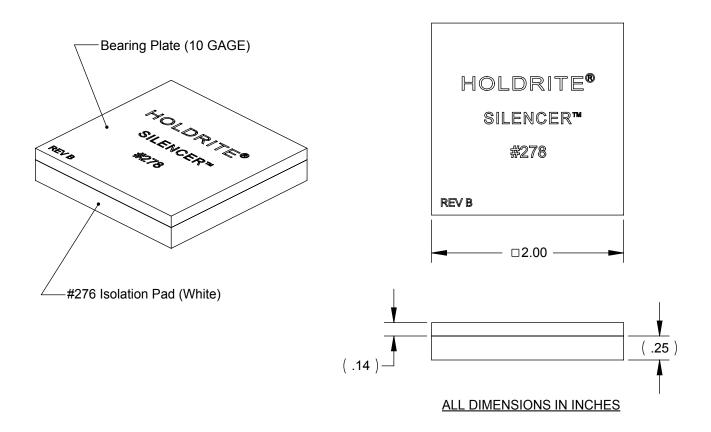
The HOLDRITE® Silencer<sup>™</sup> #278 is an engineered sound and vibration isolation pad with a steel bearing plate. Ideal for use in isolating riser clamps and equipment bases from noise transfer to the structure.
