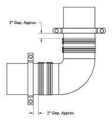
2. Position "ears" of pipe clamps perpendicular to the pipe's 90° change of direction.
