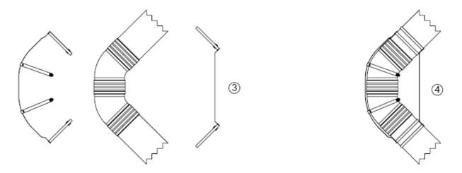
6. Position & install clamps so they are spaced between the clamps of the outside radius support and the No-Hub couplings. Do not tighten.
