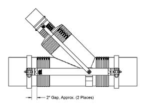
2. Position the "ears" of the two pipe clamps 90 degrees from the fitting's seam/midline.
