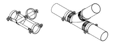
2. Position the "ears" of the three pipe clamps 90 degrees from the fitting's seam/midline.
