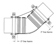
5. Position "ears" of pipe clamps perpendicular to the pipe's 45° change of direction.
