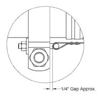
4. Prior to tightening any of the straps, place the short (1" long bolt through the hole in each strap, located at the Wye branch centerline location with the bolt threads pointing away from the fitting.
