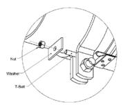
There should be a slight gap (approx. 1/4") between end of restraint and pipe clamp "ears". Adjust pipe clamp positions to achieve this gap by tapping clamps into place with a hammer.
