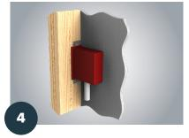
Smooth surface and corners to form the shape of the electrical box. Make sure to have the proper overlap on adjoining stud and drywall surfaces.
