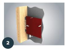
Align pad to the side of the electrical box partially overlapping the stud and adhere.
