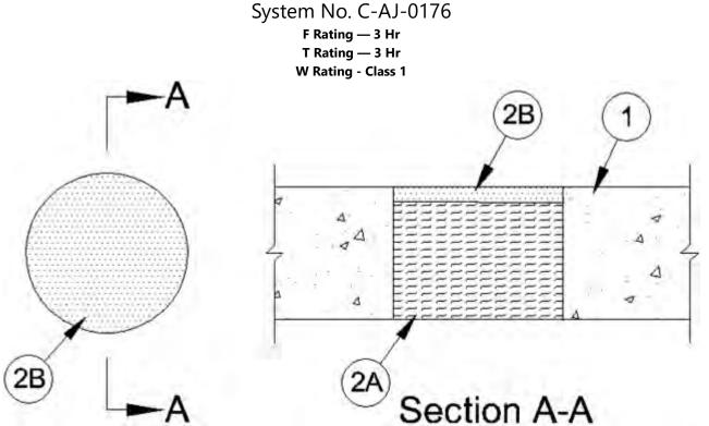
1. **Floor or Wall Assembly** — Min 4-1/2 in. (114 mm) thick reinforced lightweight or normal weight (100-150 pcf or 1600-2400 kg/m<sup>3</sup>) concrete floor or min 5 in. (127 mm) thick reinforced lightweight or normal weight concrete wall. Wall may also be constructed of any
