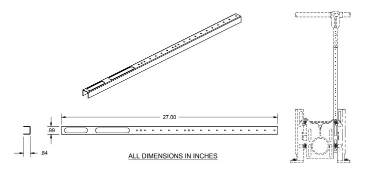
The HOLDRITE® #114-C-EXT is a Copper-Bonded<sup>™</sup> steel bracket used to extend the flushometer rough-in height of the model #114-C, #114-CO and #114-CR an additional 8-1/2" through 24-1/2". THe bracket mounts to the water closet carrier. Includes hardware for connection to the #114-C, #114-CO and #114-CR brackets.
