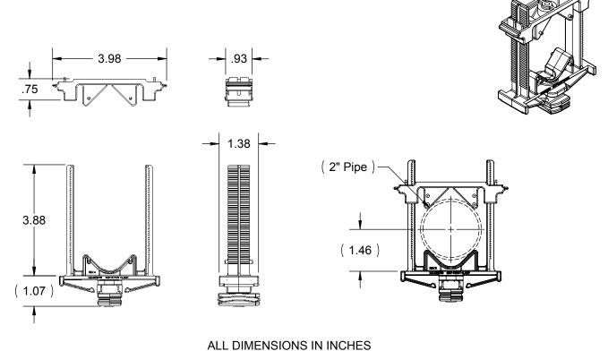
The HOLDRITE Strut Clamp™ #287-S is a flame and smoke rated variable closure clamp. Clamp supports 1" to 2" CTS/IPS tubing sizes. Supports Copper, PEX, CPVC tubing, conduit, etc. Material meets ASTM E-84 25/50 and UL94V-0 fire rating.
