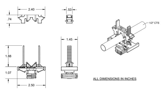
The HOLDRITE Strut Clamp™ #257-S is a flame and smoke rated variable closure clamp. Clamp supports up to 1" CTS tubing sizes. Supports Copper, PEX, CPVC tubing, conduit, etc. Material meets ASTM E-84 25/50 and UL94V-0 fire rating.
