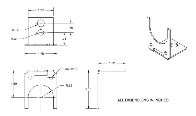
The HOLDRITE® #121 is a 16 gage galvanized steel bracket with an open "U" shape the secures single 1/2", 3/4" and 1" tubing.
