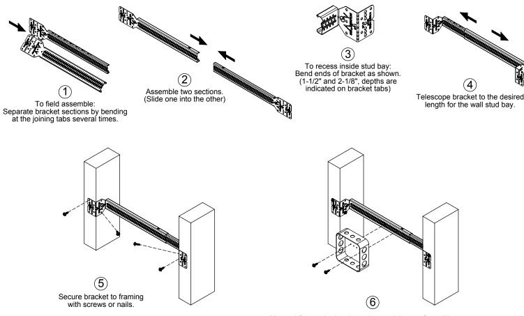
Mount J-Box to the bracket using a minimum of two (2) screws through existing mounting holes in box. #8 x 5/8" self-drilling sheet metal screws are recommended.
