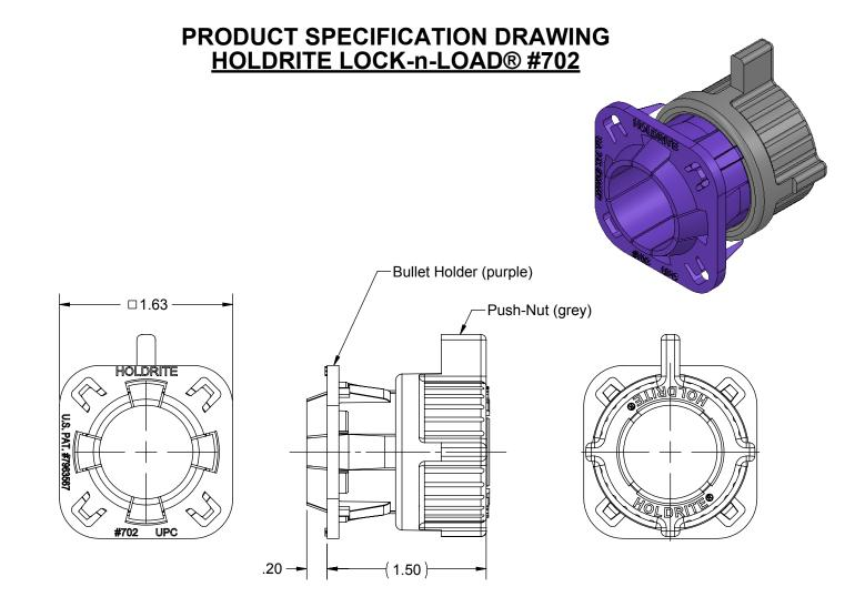
The HOLDRITE LOCK-n-LOAD® #702 is a clamp that mounts into our #103, #709, #110-R or #721 Series Brackets. This clamp requires no hardware to install and is designed to firmly grip fixture stub-outs such as bullets or similar 3/4" CTS tubing. The HOLDRITE LOCK-n-LOAD #702 is for use with PEXRITE Brackets only.
