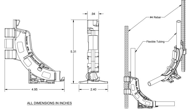
The PEXRITE® #706 supports one 3/8" - 5/8" O.D. flexible tubing line (PEX or soft copper). Ideal for positioning tubing at 90° prior to concrete slab pouring. For slab-on-grade (ground work), secure bracket with #4 rebar driven into the ground.
