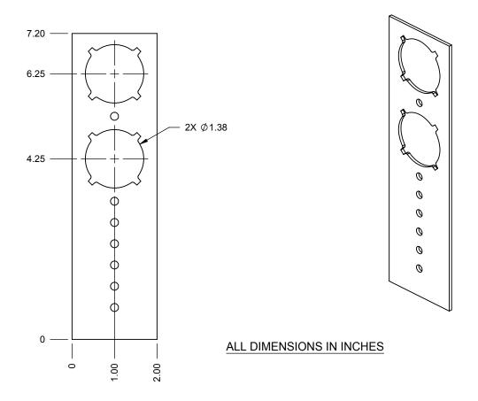
The PEXRITE® #709 is a 14 gage galvanized steel bracket with 1-3/8" keyed holes providing an approximate 4" and 6" center line off of the floor surface. Designed to work with our PEXRITE® #701 Clamp and #704 Insert. Ideal for lavatories, toilets and hose bibs. Compatible with HOLDRITE® #100 and #400 series inserts.
