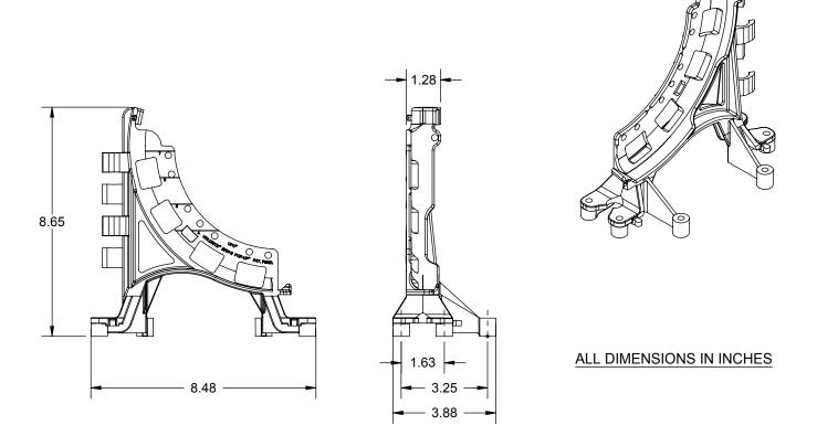
The HOLDRITE® #707-E POP-UP<sup>™</sup> supports flexible pipe and tubing lines or rigid conduit up to 1-1/4" IPS in a 90° pattern. Ideal for positioning in-slab piping prior to concrete slab pouring. For elevated slabs, nail or screw bracket to form decking or edge form. For slab-on-grade (ground work), secure bracket with #4 rebar driven into the ground. Piping is attached to bracket with zip ties (3 included).
