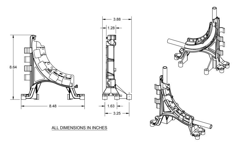
The PEXRITE® #707 POP-UP™ supports one 3/8" - 7/8" O.D. flexible tubing line (PEX or softer copper). Ideal for positioning tubing prior to concrete slab pouring. For elevated slabs, nail bracket to form decking or edge form. For slab-on-grade (ground work), secure bracket with #4 rebar driven into the ground.
