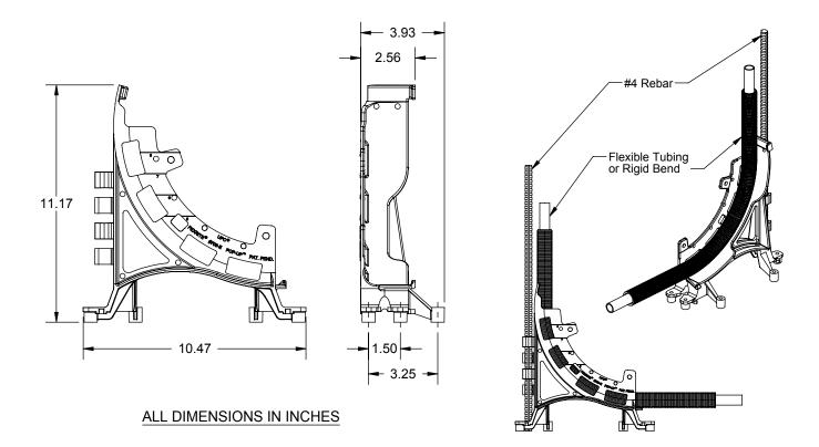
The PEXRITE® #708-E POP-UP™ supports flexible pipe and tubing lines or rigid conduit up to 2" in a 90° pattern. Ideal for positioning pipe prior to concrete slab pouring. For elevated slabs, nail bracket to form decking or edge form. For slab-on-grade (ground work), secure bracket with #4 rebar driven into the ground.
