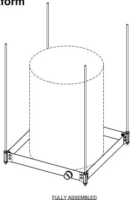
The Suspended Water Heater Platform is engineered to support water heaters up to 20 U.S. gallons (up to 375 pounds total weight). This time and labor savings tool is designed for the Professional Contractor. Design features requested by plumbers are incorporated into a professional platform that can be suspended with all thread rod. See Installation Instructions for detail.
