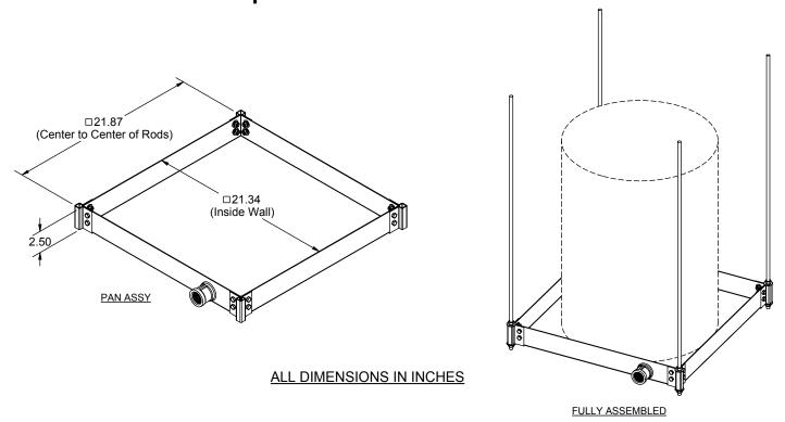
The Suspended Water Heater Platform is engineered to support water heaters up to 20 U.S. gallons (up to 375 pounds total weight). This time and labor savings tool is designed for the Professional Contractor. Design features requested by plumbers are incorporated into a professional platform that can be suspended with all thread rod. See Installation Instructions for detail.
