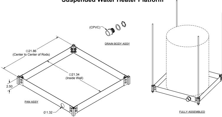
The Suspended Water Heater Platform is engineered to support water heaters up to 20 U.S. gallons (up to 375 pounds total weight). This time and labor savings tool is designed for the Professional Contractor. Design features requested by plumbers are incorporated into a professional platform that can be suspended with all thread rod. See Installation Instructions for detail.
