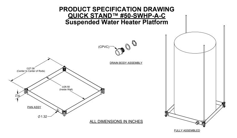
The Suspended Water Heater Platform is engineered to support water heaters up to 50 U.S. gallons (up to 600 pounds total weight). This time and labor savings tool is designed for the Professional Contractor. Design features requested by plumbers are incorporated into a professional platform that can be suspended with all thread rod. See Installation Instructions for detail.
