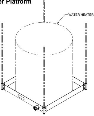
The #60-SWHP-M Suspended Water Heater Platform is engineered to support water heaters up to 50 U.S. gallons, or other equipment, up to 750 pounds total weight. This time and labor savings tool is designed for the Professional Contractor. Design features requested by plumbers are incorporated into a professional platform and drain pan combination that can be suspended with 3/8" or 1/2" all thread rods. See Installation Instructions for detail.
