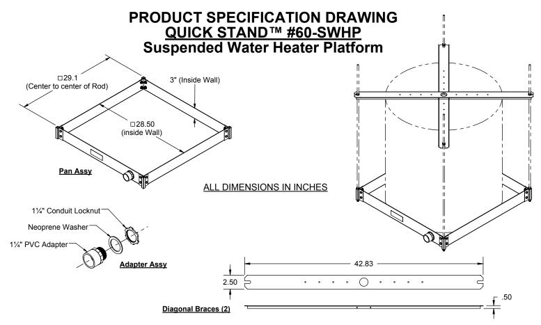
The #60-SWHP Suspended Water Heater Platform is engineered to support water heaters up to 50 U.S. gallons, or other equipment, up to 750 pounds total weight. This time and labor savings tool is designed for the Professional Contractor. Design features requested by plumbers are incorporated into a professional platform and drain pan combination that can be suspended with 3/8" or 1/2" all thread rods. See Installation Instructions for detail.
