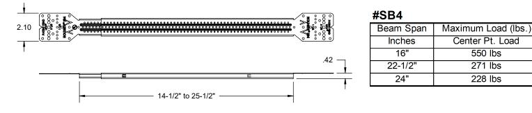
Hole pattern permits attachment of a wide variety of Clamps, Fittings, J-Boxes, Outlet Boxes, etc. The wide face provides excellent stability and is also ideal for attachment of both 2-eared and 3-eared shower head and tub spout 90°s. Bracket attaches between studs in span from 10-1/4" through 25-1/2" (depending on model #). End tabs bend easily at 3/4", 1-1/2" & 2-1/4" for in-wall set backs. Optional nailer tabs can be used for quick attachment to wood studs for positioning purposes.
