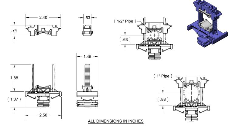
The HOLDRITE® Acoustical Strut Clamp™ #257-P is a strong, sound rated variable closure clamp. Two acoustical inserts isolate the pipe from the support structure, reducing piping noise and vibration, while allowing normal pipe expansion and contraction. Clamp supports up to 1" CTS tubing sizes. Supports Copper, PEX, CPVC tubing, conduit, etc. Framework complies with UL94V-2 fire rating.
