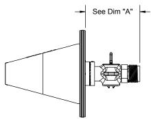
The TESTRITE® TRW2V through TRW6V (TEST WEDGES with VALVES) are used in conjunction with TESTRITE TEE'S, which allow temporary blocking of the DWV stack for testing while providing connections for convenient system fill and drain. Available in 2", 3", 4" & 6" piping systems.
