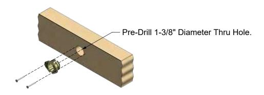
INSERT 2 NAILS TO THROUGH STUD TO SECURE TO FRAMING. (FIG. 1)
