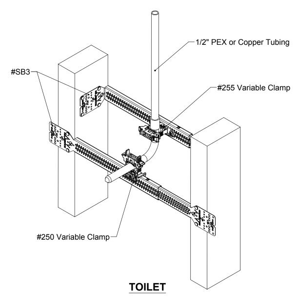
SHOWN WITH HOLDRITE® #250 & #255 STOUT CLAMPS™ WITH ACOUSTICAL PADS MOUNTED ON HOLDRITE #SB3 STOUT BRACKETS™ WITH SCREWS. THESE CLAMPS ACCEPT 3/8" THROUGH 1" TUBING. (#250-S & #255-S CLAMPS AVAILABLE FOR 25/50 PLENUM RATED APPLICATIONS) (#SB3 FITS 10 1/4" - 17 1/2" STUD BAYS; #SB4 FITS 15 1/4" - 25 1/2" STUD BAYS).
